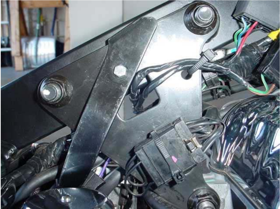
Carb Brace – Side View, Installed
