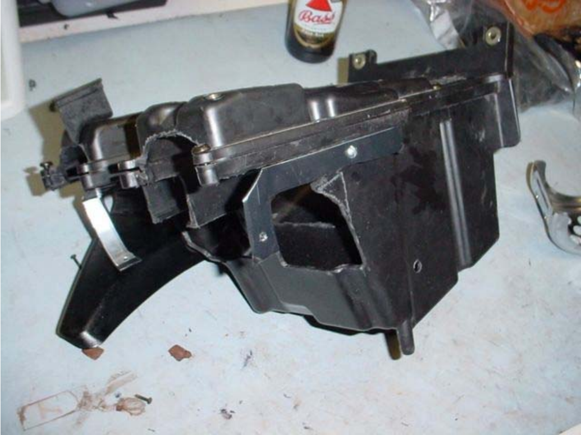
Left side brace covered with tape and installed after airbox cutting
