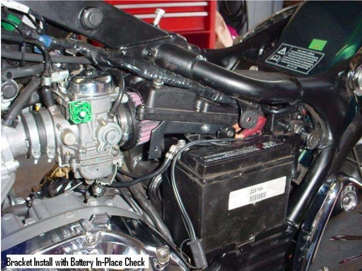
Verifying Bracket Installation/Removal with Battery In-Place
