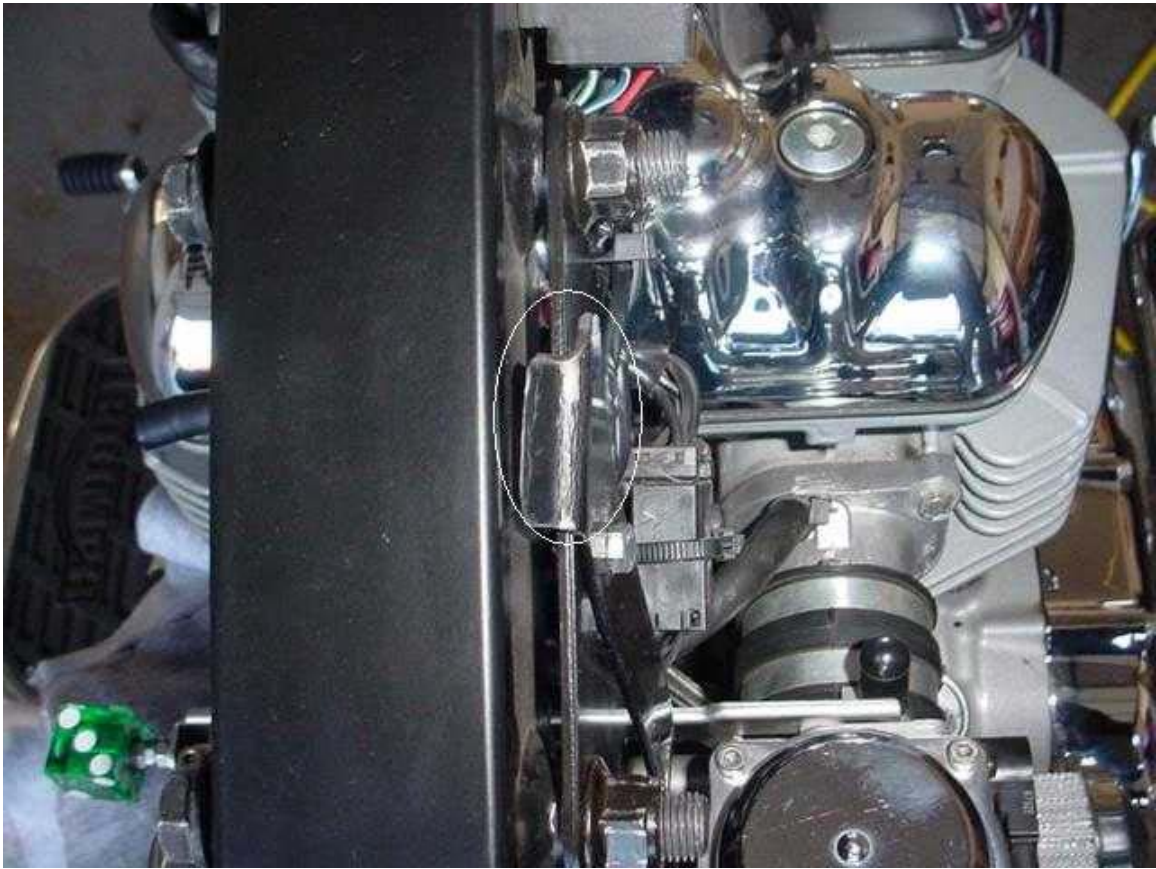
Carb Brace – Tope View, Installed
