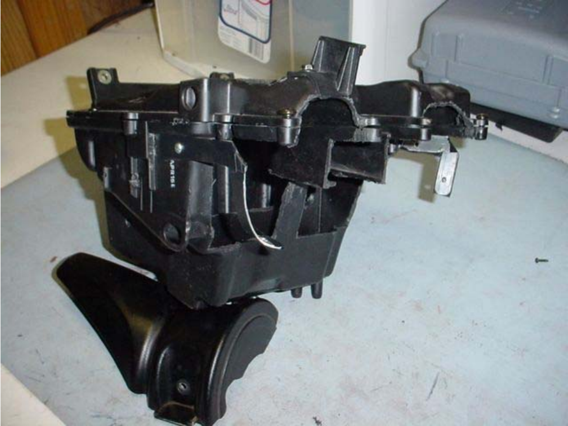
Right side brace covered with tape and installed after airbox cutting
