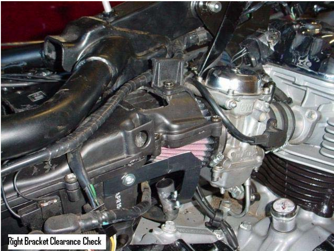
Verifying Right Bracket Clearance
