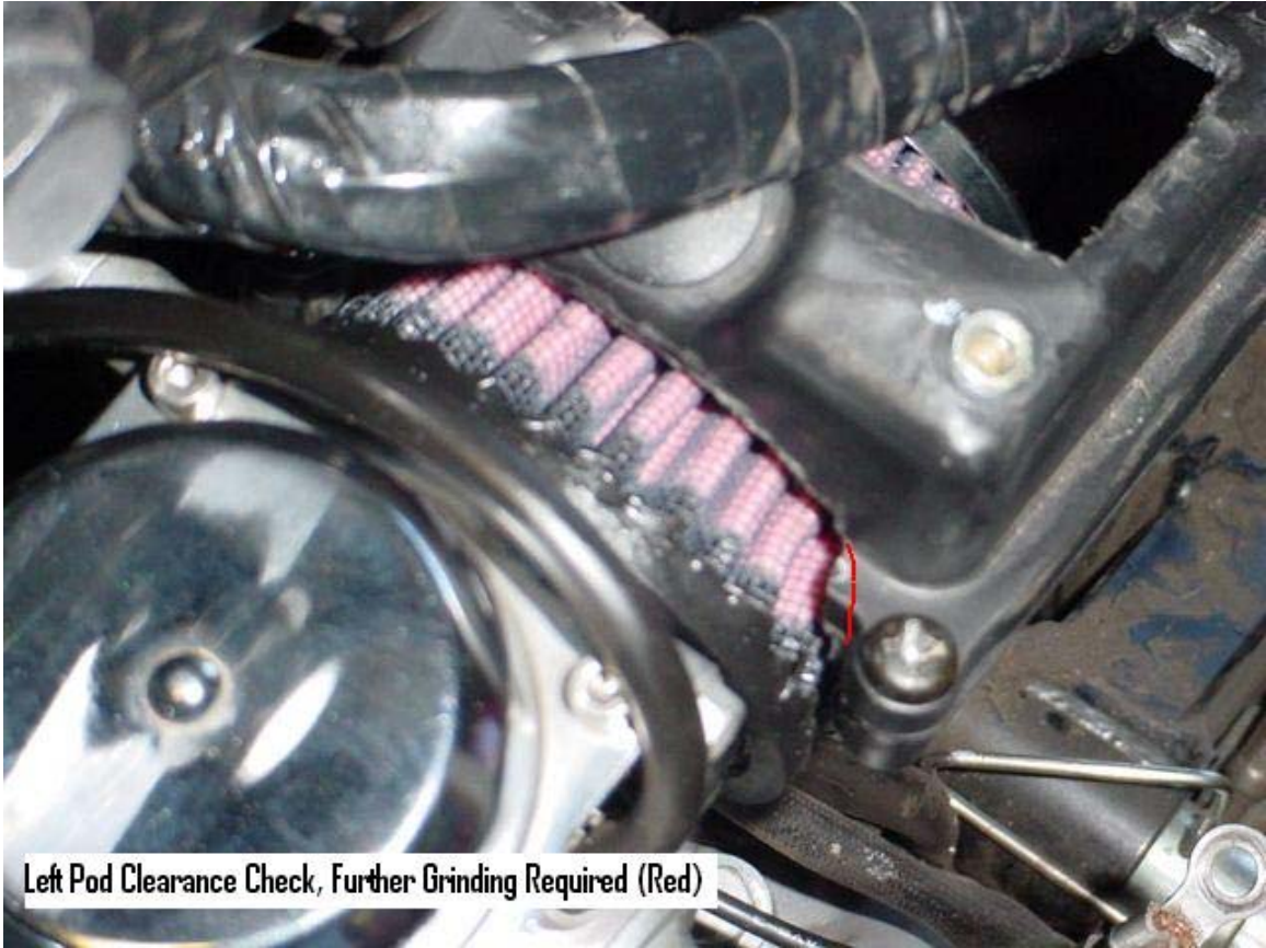
Verifying Left Pod Clearance
